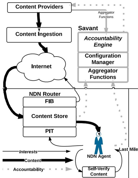
Figure 1: The NDN architecture with the Savant framework.
