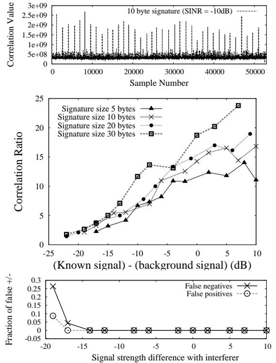
**Figure 6: (a) The correlation value spikes every time a known signature arrives amid a background transmission. (b) Correlation Ratio with varying transmitter-receiver separation and signature size. (c) False positive and false negative rates of discerning collision notification against varying transmitter-receiver separation.**
