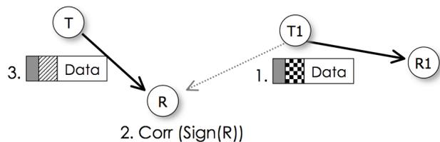
Figure 4: Under interference, R correlates its own signature, denoted as Corr(Sign(R)).
