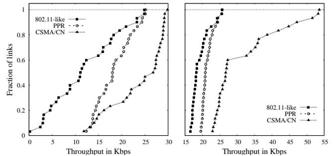
**Figure 9: (a) CDF of throughput in Kbps where all nodes are continuously active. (b) CDF of throughput in Kbps with fixed size traffic (like FTP).**
