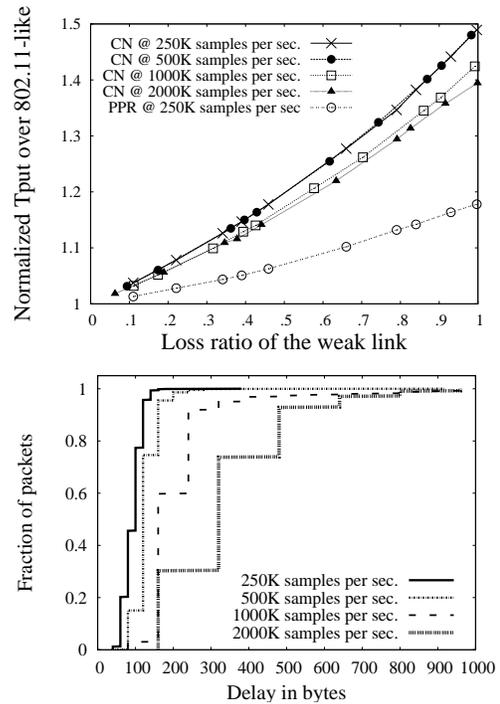
**Figure 8: (a) Performance gains with CSMA/CN and PPR over packet receivers (b) CDF of notification overhead for CSMA/CN in bytes**
