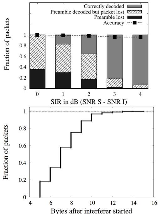
**Figure 7: (a) Collision detection accuracy with increasing interference strength (b) CDF of bytes when the collision was detected after it started**
