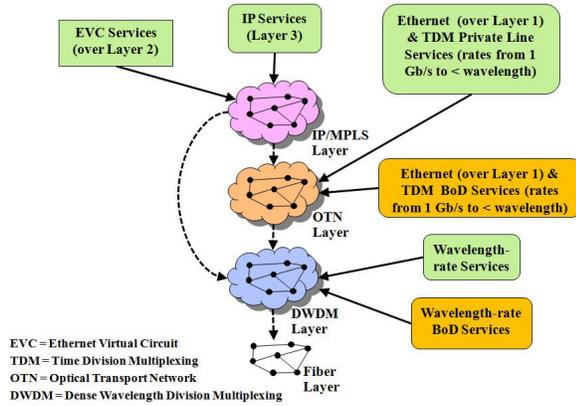
Figure 2: Carrier's view of future services & network layers.
