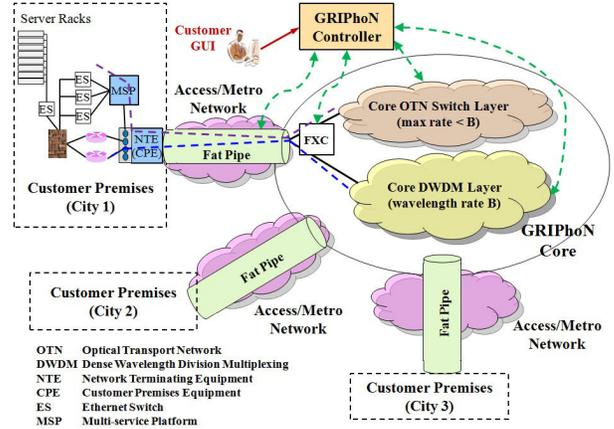
Figure 3: BoD for inter-data center communication using GRIPhoN.
