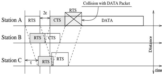
Fig. 3. MACA unsafe transmission:
