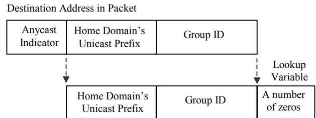
Figure 6: Mapping an unpopular anycast group to a unicast address in the home domain. The anycast destination is assigned to a lookup variable. The anycast indicator is shifted off the variable, then the variable is looked up in the router's unicast routing table. The anycast packet remains intact.
