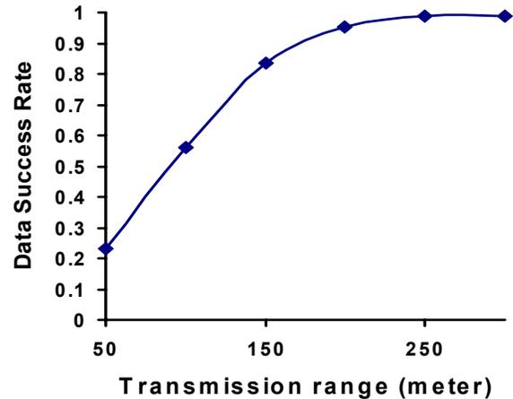
**Figure 2. Data success rate as a function of the transmission range. Resource report size = 64bytes; vehicular density = 40 vehicles/ sq.km**
