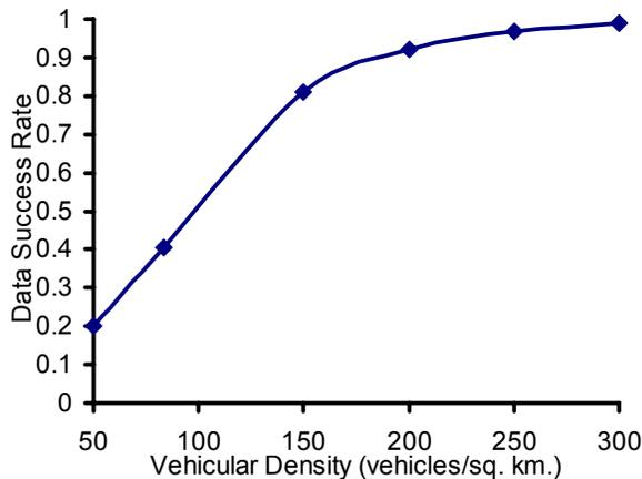
**Figure 1. Data success rate as a function of the number of nodes. Resource report size = 64bytes; transmission range = 150m.**
