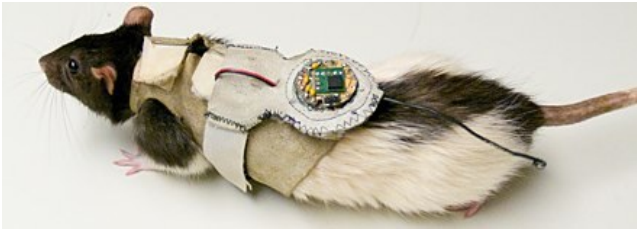
Figure 1: Norway rat equipped with sensor node
