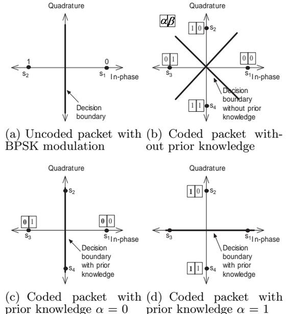
Figure 1: Signal space and decision boundary with and without physical layer network coding
