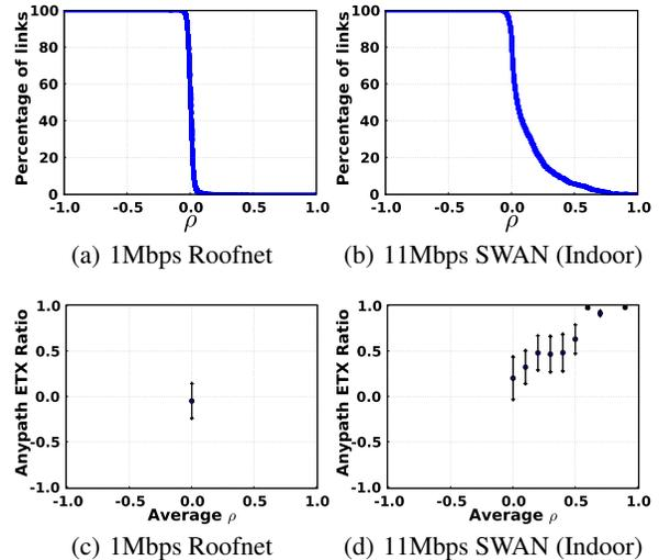
Figure 2:  $\rho$  and opportunistic routing. @1Mbps, none of the Roofnet receivers have reception dependent on reception at other receivers. @11Mbps, about 5% of the SWAN receivers have dependent reception. As the average  $\rho$  of all receiver pairs in an anypath increases, the anypath ETX ratio also increases; if many receiver pairs have correlated reception, the anypath ETX estimate (assuming independent receivers) and the actual anypath ETX are very different.
