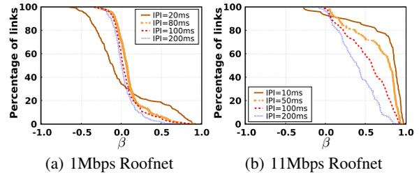
Figure 1:  $\beta$  for Roofnet. 1Mbps links have mostly low  $\beta$ 's while 11Mbps links have high  $\beta$ 's.
