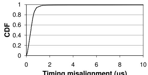
**Figure 12: CDF of symbol timing mismatch with broadcasting.**
