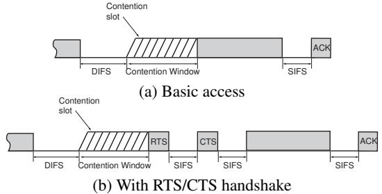
**Figure 1: Illustration of CSMA/CA access method.**
