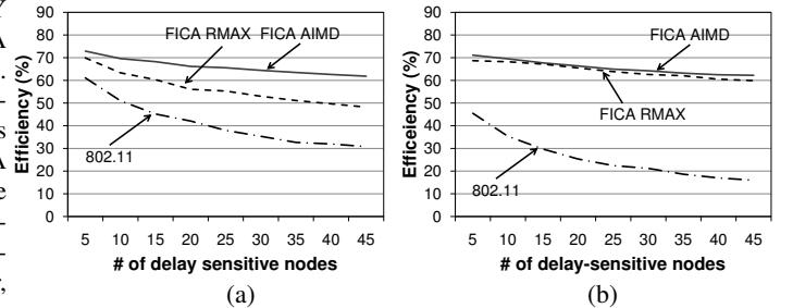
**Figure 10: Mixed traffic. Five nodes are fully saturated. All other nodes have delay-sensitive traffic with a uniform distribution between 800Kbps to 5Mbps. (a) 802.11 PHY 150Mbps; FICA 145Mbps. (b) 802.11 PHY 600Mbps; FICA 580Mbps.**
