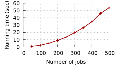
Figure 5: Running time of the offline planner heuristic in Corral for a 4000 machine cluster with varying number of jobs.
