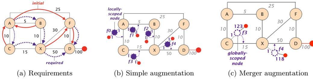
**Figure 6: Outcome of our per-destination augmentation algorithms. Simple produces larger topologies (with locally-scoped lies) in a very short time, while Merger reduces the size of the augmentation by relying on globally-scoped lies and a longer computation.**
