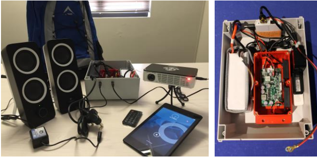
Figure 2: Cinema-in-a-backpack system (left) and mobile infostation (right).
