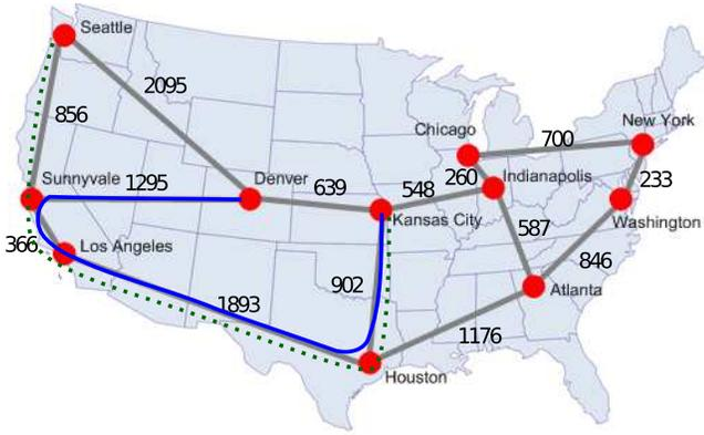
**Figure 2:** This figure shows examples of the NotVia protection paths in the Abilene topology. The numbers next to a link are link costs. The solid line shows the protection path from Denver to reach Kansas City when the link to Kansas City fails, and the dotted line shows the protection path from Seattle to Kansas City when the Denver node fails.
