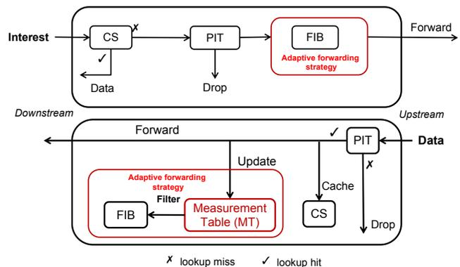
Figure 1: Optimized NDN forwarding pipelines with an adaptive forwarding strategy: bind Measurement Table to PIT
