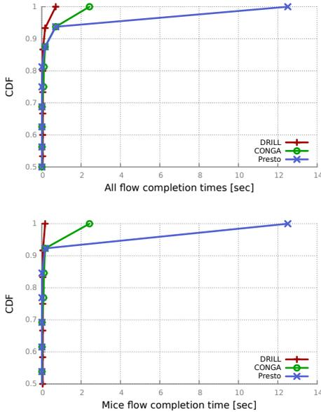
Figure 4: Flow completion time in an incast scenario.
