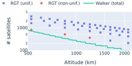
**Figure 1: Minimum number of satellites required to cover a single repeat ground-track compared to number of satellites required for uniform global coverage in a Walker-delta constellation at 65° inclination.**
