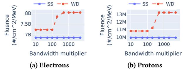
**Figure 10: Estimated median radiation exposure over one day for a satellite in the constellations evaluated in Figure 9.**
