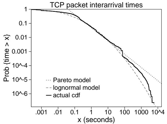
Fig. 9. ccdf of interarrival times for TCP packets.
