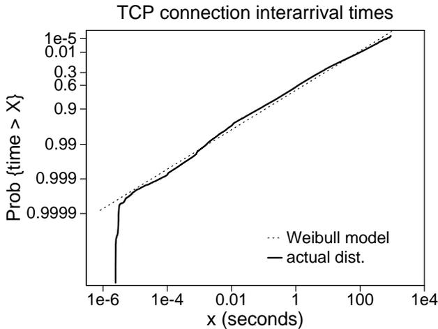
Fig. 11. Weibull test for TCP connection interarrivals.
