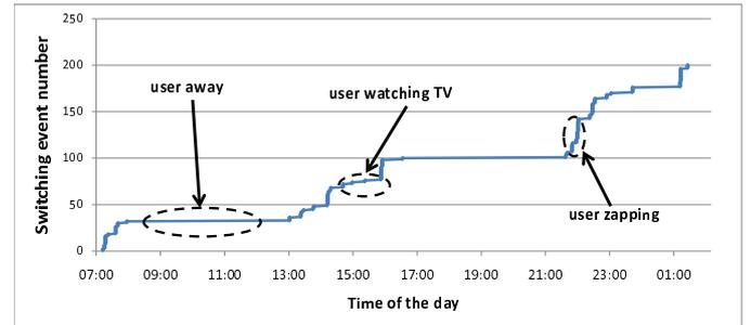
Figure 1: IPTV switching events (one typical user, one typical day)
