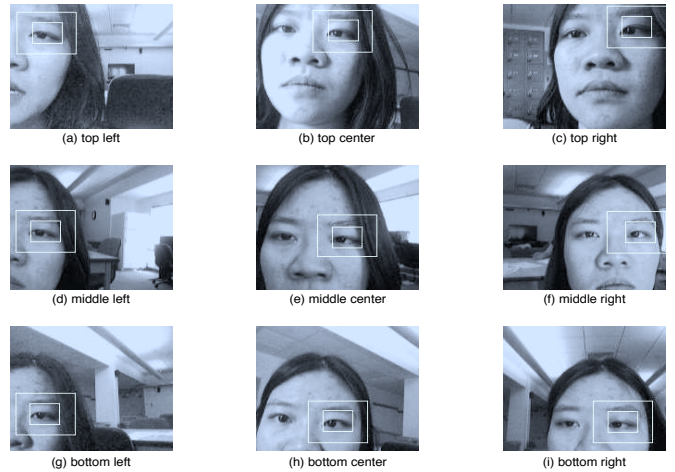
Figure 2: Eye capture using the Nokia N810 front camera running the EyePhone system. The inner white box surrounding the right eye is used to discriminate the nine positions of the eye on the phone’s display. The outer box encloses the template matching region.
