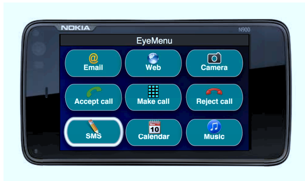
Figure 4: EyeMenu on the Nokia N900. While looking the display, a button is highlighted if it matches the eye position on the display. The highlighted button is ready to be “clicked” with a blink of the eye. In this example, the user is looking at the SMS button and the SMS keypad is launched by blinking the eye.
