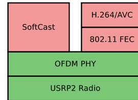
**Figure 1** The architecture of the experiment. We compare the joint design of SoftCast to the standard design using H.264/AVC on top of the 802.11 FEC. Both schemes use the same OFDM PHY and the USRP2 radio front-end.
