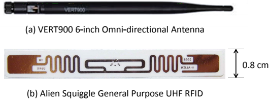
Figure 7—Antenna and commercial UHF RFID used in experiments: (a) We use the VERT900 6-inch vertical antenna as PinIt’s moving antenna. (b) the Alien Squiggle General Purpose UHF RFID Tags. Note that the sizes of (a) and (b) are not proportional to the real sizes of the devices.
