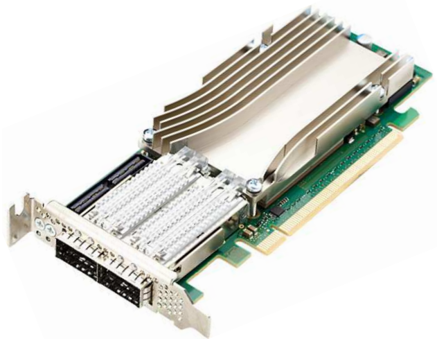
Figure 1: Front view of the NFB-200G2QL FPGA card.
