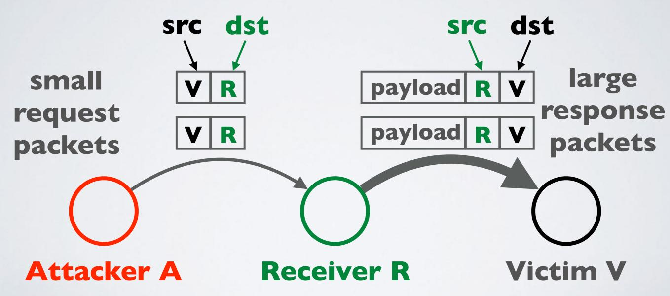
Volumetric Reflection-Amplification Attack
