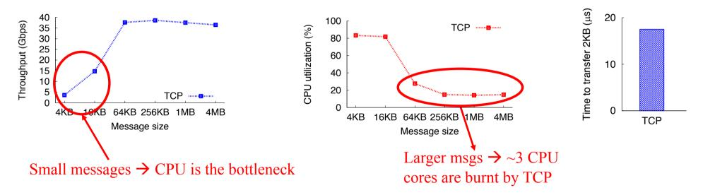
The above test was done on Windows machines [DCQCN, SIGCOMM'15]; Linux machines show a similar trend [Sandstorm, SIGCOMM'14]
