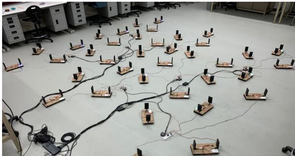
**Figure 10:** A floor testbed of 38 simple elements.
