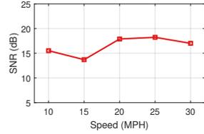
Figure 18: Impact of vehicle speed.
