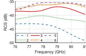
**Figure 3: RCS with different number of antenna pairs.**
