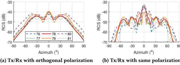
**Figure 6: RCS of PSVAA across the 76-81 GHz frequency band.**
