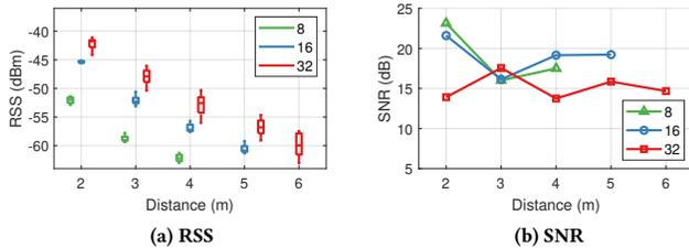
Figure 15: Impact of radar-to-tag distance.
