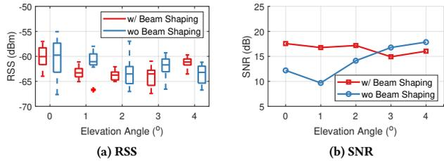
Figure 14: Effectiveness of elevation beam shaping.
