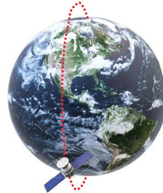
**Figure 1: Earth observation satellites typically operate in polar low-earth orbits. As the Earth rotates under them, they scan different parts of the Earth during each orbit. A single satellite may image the Earth across several days, so operators plan to rely on large constellations to achieve collective imaging frequency of minutes to hours.**
