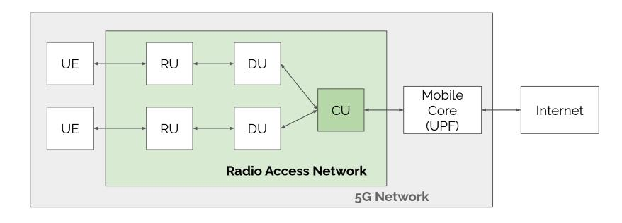
CU- Central Unit; DU- Distributed Unit; RU- Radio Unit; UPF- User Plane Function UE- User Equipment
